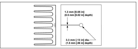
Figure 5-3. Zero Degree Angle Attach Methodology (Top View)
